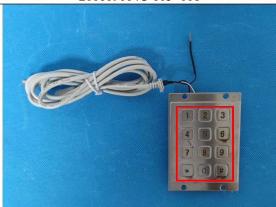
210609004C-001 Red rust appears
